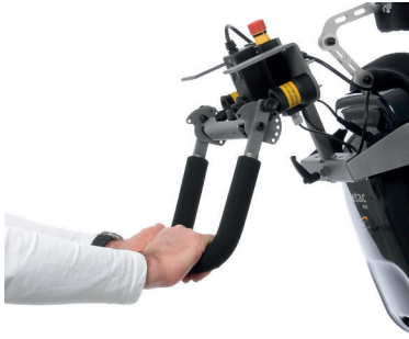
Figure 3. Correct use of attendant control in order to avoid the risk of getting trapped
